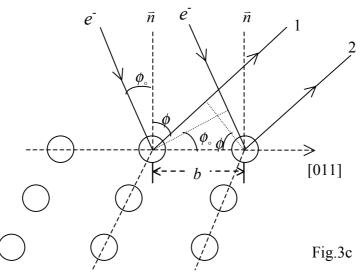
The path difference between electron beam 1 and 2 is
