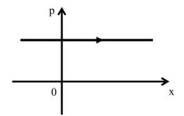
Fig. 1. Phase trajectory of a free particle.
