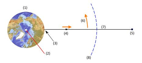
**Figure 1.** Space Elevator (adapted from wikipedia).(1) Earth; (2) North pole; (3) Anchored at equator; (4) Climber; (5) Counterweight; (6) Rotates with Earth; (7) Cable; (8) Geostationary orbit altitude.
