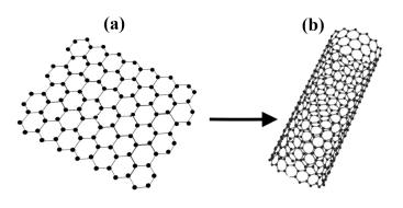
Figure 3. Graphene (a) and carbon nanotube (b).
