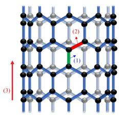
**Figure 5.** An illustration of a carbon nanotube with 9 carbon-carbon parallel bondings. Note: In this problem, there are 27 carbon-carbon parallel bondings. (1) parallel bond; (2) slanted bond; (3) tube axis.
